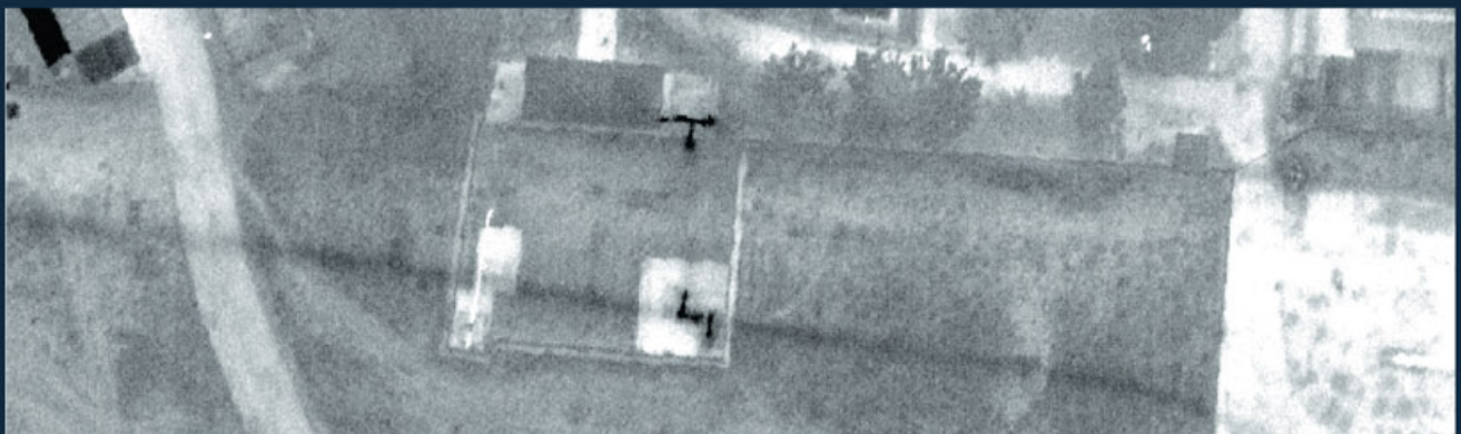
Underground ammonia pipe. Temperature difference between pipe and environment - 5°C. Temperature difference on ground surface - 0,5°C.
